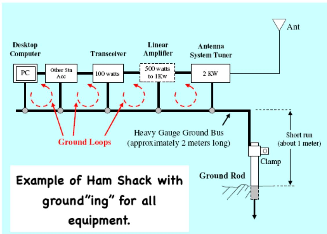
In this example, the grounded power connection for each piece of equipment provides a separate path to a different grounding rod at the electrical panel, (power connections not shown). The issue could be exasperated by powering equipment from different circuits.
